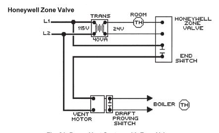
Fig. 21: Power Vent System with Zone Valve
